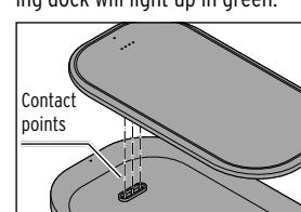
3. Place the power bank on the charging dock as illustrated. The contact points on the power bank and on the charging dock must be facing each other.
